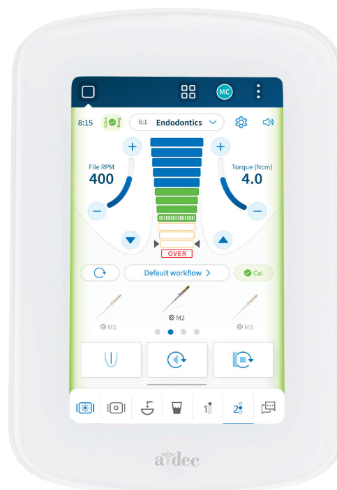
Get real-time guidance as you approach the apex with clear step tracking and performance metrics. (Interface as shown on A-dec 500 Pro DS7 screen.)
